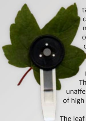
takes place. The body of the clips are constructed from white plastic to minimise the effects of heat build-up on the leaf during the period when the clip is in place. The locating ring section of the clip which interfaces with the fluorimeter optical assembly is constructed from black plastic. This ensures that the measurement is unaffected when measuring during conditions of high ambient light intensity.
