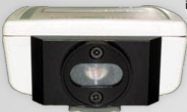
The detector is a highly sensitive PIN photodiode and associated amplifier circuit. The optical design and filtering ensure that it responds maximally to the longer wavelength fluorescence signal and blocks the reflected shorter wavelength LED light used as the source of illumination. The entire optical assembly is sealed behind a clear glass window which creates a barrier against moisture and dirt which are inherent problems for field based instruments.
